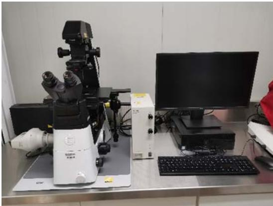
Microscopio Ti2 (Nikon) y Phmetro/iometro/ORP SevenCompact (Mettler Toledo).
